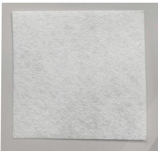
Fig. 1: Procedure A: Particle filter Nissan 272774BR1A, filter medium; test specimen at the end of the test period (example);rating: 0
